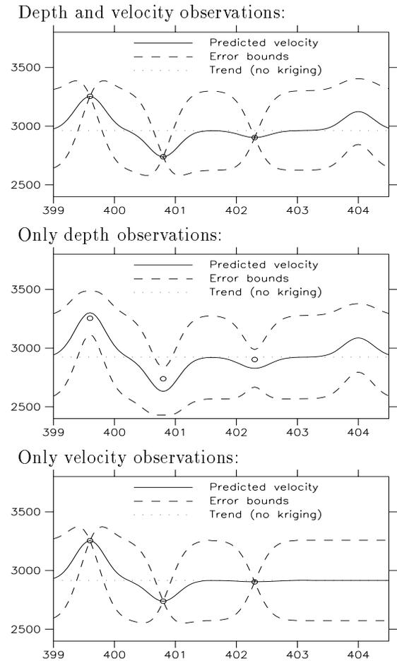
Figure 8: Bayesian velocity predictions for interval between Top and Base.
