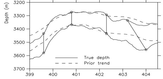
Figure 2: Possible true depth to Top and Base. Dashed lines are prior guesses. Depth observations are shown as small circles.
