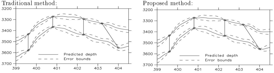
Figure 4: Predicted depth to Top and Base. Notice the failure of the traditional approach at the deviating well.
