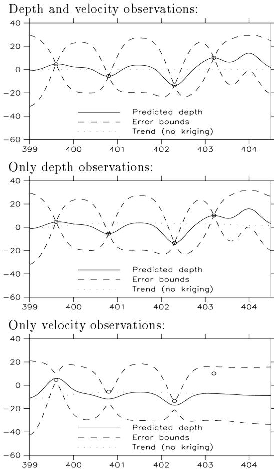
Figure 7: Bayesian depth predictions for Top. The trend for predictions with both depth and velocity data has been subtracted to exaggerate the local influence of the data.
